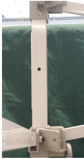
Figure 2: Position of Drilled hole in EZ-up frame.
